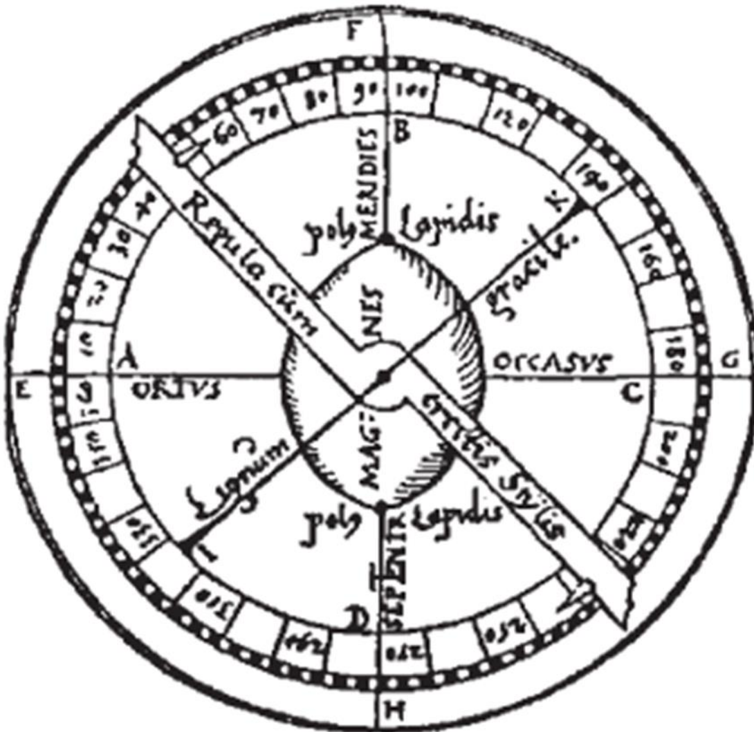
Fig. 1.1. One of Petrus Peregrinus' inventions is this "Astrolabium", an oval lodestone mounted inside a wooden box. The four points of the compass and 360 subunits were painted on the inside of the box. This instrument was placed in a bowl of water to determine the azimuth of the sun, for example, and the angle was read after the astrolabium had stopped moving.
