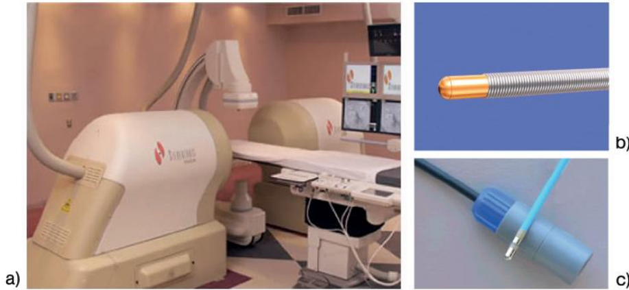
Fig. 1.8. (a) The Niobe3 system, a magnetic navigation system built by Stereotaxis Inc., St. Louis, Missouri, USA. The system is based on two large permanent magnets that, upon proper rotation and movement, are able to precisely direct a magnet-tipped guide wire (b) or electrophysiology mapping catheter (c) within the patient's vascular system. This system was approved by the FDA in the USA in 2003 for multiple interventional cardiology and electrophysiology procedures.
